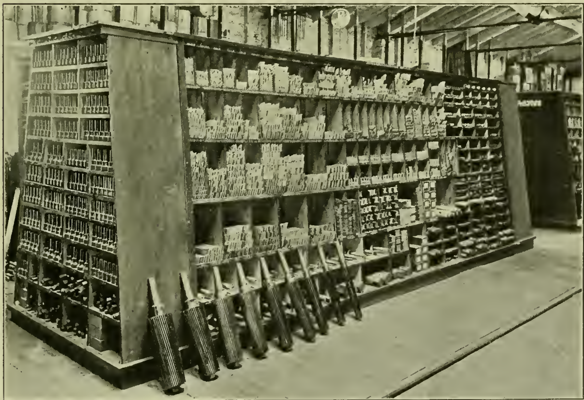
FIG. 12.—GENERAL STOREHOUSE STOCK OF STANDARD TOOLS MANUFACTURED IN TOOL ROOM AT TOPEKA AND SUBJECT TO REQUISITION FROM ALL OUTLYING SHOPS.
